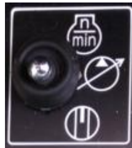
Pump Control Selector Switch
